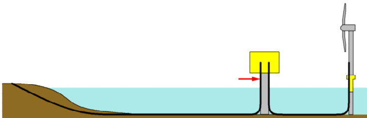
Figure 13. Example of long length installation with water with steep uphill section at the end
